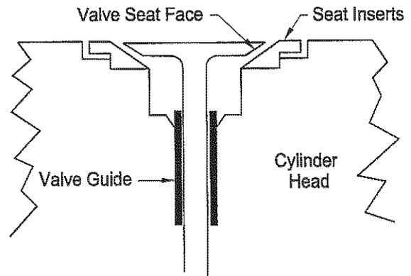
**Fig. 8: Shows an exhaust valve, seat and guide.**
