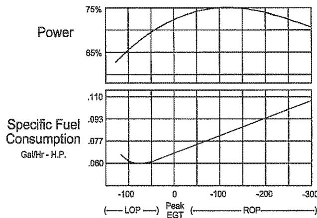
**Fig. 6: Typical power curve and specific fuel consumption for most aircraft engines.**
