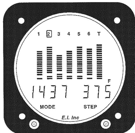
Fig. 18: Shows Normal mode with the engine running lean.
