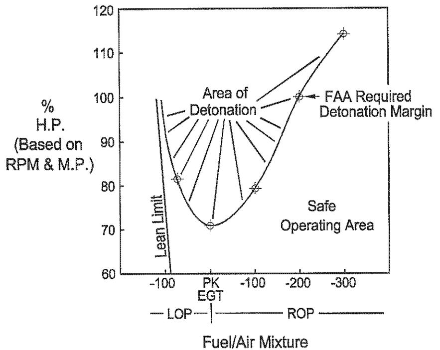
Fig. 13: Operating envelope for an aircraft engine set to the FAA required detonation margin with normal cylinder turbulence.
