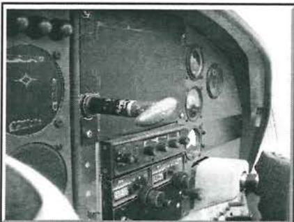
Panel-mounted tow release handle in a Soccata Rallye.
